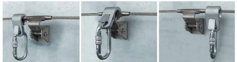
Sequence for travelling the slide, a movable anchor point, along the system including passing through a lug without hampering the fall protection capability
