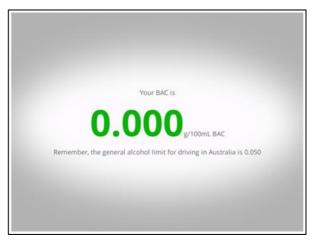
If the BAC detected is zero, the display will be green; from 0.001 to 0.050g/100ml, the display will be orange and for readings above 0.050g/100ml, the display will be red.
