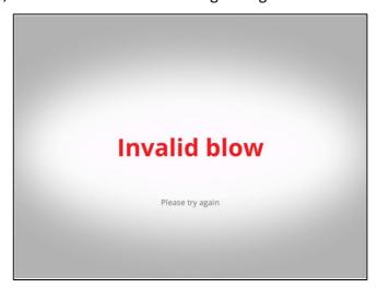
If the blow is invalid, cease blowing, wait until the Insert Straw and Blow screen is displayed and then provide another sample.
