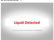
It is possible that liquid has been blown into the sample port. Ensure liquid is not present and try again. If the problem persists, allow a suitable time period for the liquid to clear itself (anywhere up to 48hrs), or refer to section 5.2 of this manual. If the problem persists, contact Alcolizer on 1300 789 908.
