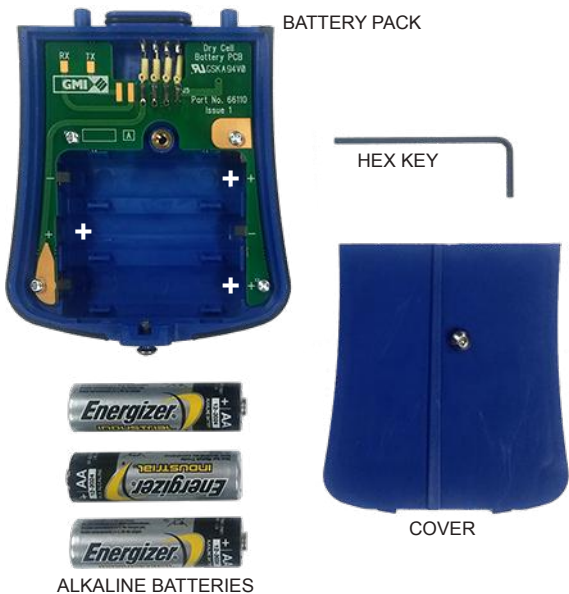
Fig. 4.13 Alkaline Batteries Removed
