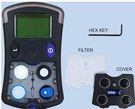
Fig. 4.2 Filter and Cover Removed
