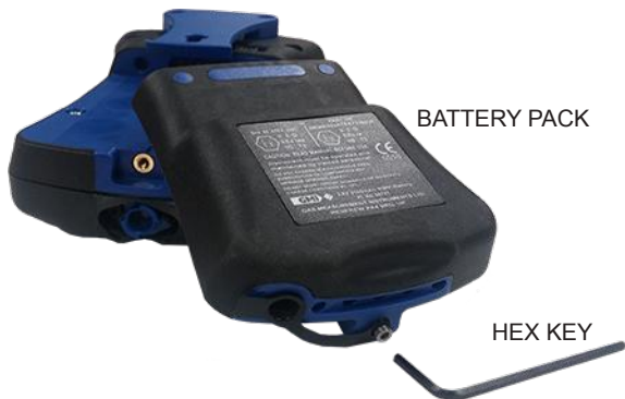
Fig. 4.11 Battery Pack Removed
