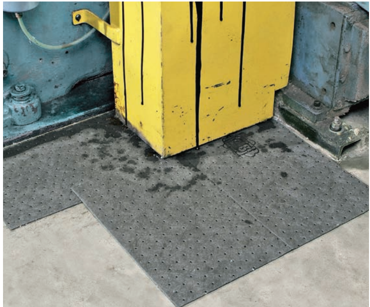
Absorbent mat pads are a great way to control machine leaks.
