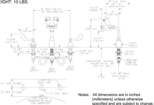
**IMPORTANT:** The supply line for plumbed units shall provide an uninterruptible supply of flushing fluid at a minimum of 30 psi . of flow pressure. If shut off valve are installed in the supply line of the eyewash for maintenance purposes, provisions shall be made to prevent unauthorized shut off.
