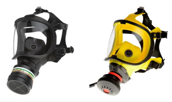
Newly designed, extra wide view full face mask complying to European norms EN 136 - Class 3. One size fits all. For use with dust, gas and combined filters with a threaded connector conforming to EN 148/1 and an overpressure version for use with compressed air supply devices, according to EN 148/3. All versions are available in EPDM and silicone rubber.
