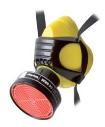
The **Polimask 2000 Alfa** is a one size half mask, available in EDPM and silicone rubber, complying with EN 140. **The Polimask Alfa** is equipped with standard screw in connector according to EN 148/1 for use with one **DIRIN series filter**.
