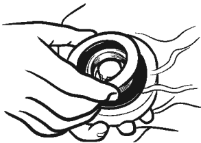
Fig. 4. Fit plastic washer
