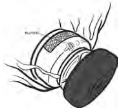
Fig. 7. Position of RED LED
