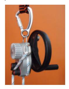
The handwheel can be rotated to elevate the accident victim till he/she can either be lifted to a secure base or the securing lanyard of the person to be rescued can be detached. When doing so, the slack rope between the turning device and the cam cleat is pulled downward and tightened over and over again. This helps in minimising the distance over which the person to be rescued may slip in case the handwheel is inadvertently released.
