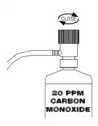
THE MONITOR IS NOW CALIBRATED AND SHOULD BE RECALIBRATED MONTHLY OR IF ACCURACY IS QUESTIONABLE. CHECK LOCAL REQUIREMENTS AND RECALIBRATE AS REQUIRED.
