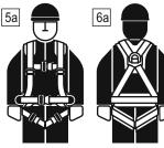
Work "positioning" belt must be at the waist height. Buckles must be arranged symmetrically on both sides.
