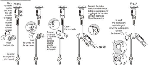
The AC080 device used for arresting the fall should be attached only to the cogging point of the harness compliant with EN 361. The cogging point must be marked with letter 'A' Fig. B
