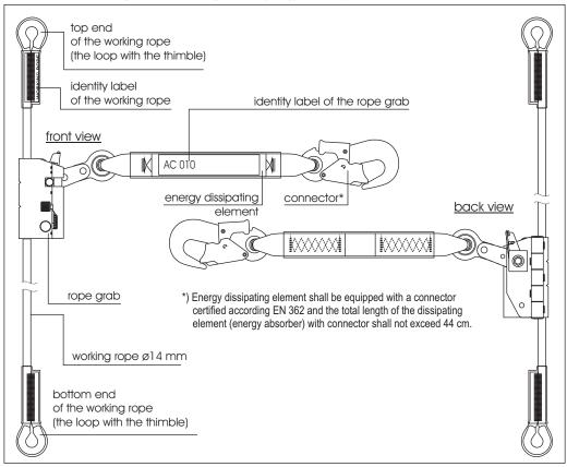
Using the AC 010 fall arrester in connection with fall arrest system must be compatible with use instructions of the fall arrest systems and obligatory standards:
