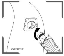
Insert the externally threaded end of the breathing tube into the inlet hole and tighten the breathing tube into the inlet until tight making sure not to twist the hood as it gets tight.
