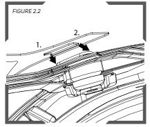
Line up the tabs of the lens with the clips on the sides of the helmet. 1. Slide the 1st side under the front side of the clip and slide back. 2. Snap the 2nd side of over the back of the clip.
