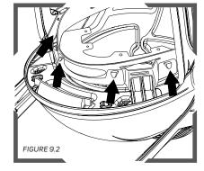
Replace the brow pad by placing the holes on one side over the hooks on the head harness and then wrap the pad over the top of the head harness. Stretch the pad around the bottom of the head harness and secure the holes over the hooks.
