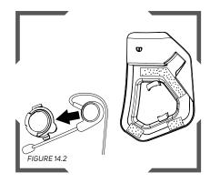
Place the Communication ear piece into the attachment clip. Then attach the Communication Clip into the slots on the inside of the cover.
