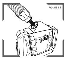
Insert the bayonet end of the breathing tube into the outlet of the PX4 AIR® PAPR and twist it in until it is secure.
