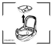
The comfort pad is attached to the inside of the Impact Liner with hook and loop. Pull the comfort pad out of the helmet.
