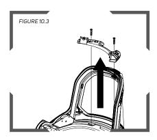
To remove the Impact Liner, remove the head harness bracket by removing the screws holding it in place.
