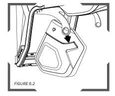
Slide the ends of the head harness into the slots on the side pad covers and reattach the head harness ratchet.
