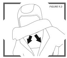
Tuck the inner bib into the collar of your shirt, coveralls, or protective gear to prevent contaminants from entering the hood. Pull the outer hib down.
