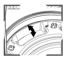
Airflow can be directed by positioning the air flow director so that the air flows more towards the visor or towards the face.
