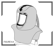
With air flowing through the respirator adjust the air pressure at the point of attachment to the recommended pressure as specified in the Breathing Air Pressure Table (page 14).
