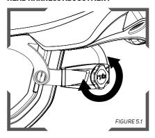
The head harness can be tightened or loosened using the ratchet knob on the back of the headband.
