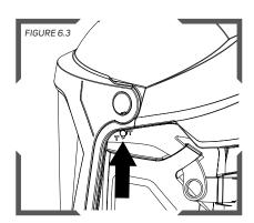
Slide the tab on the side pad covers into one of the three T-shaped slots in the head harness depending on the desired height of the side pads. Reinsert the ratchet pivot points.
