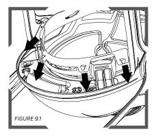
To remove the brow pad, stretch the brow pad over the hooks on the head harness and take it off. Clean it with mild detergent or replace it with a new one.
