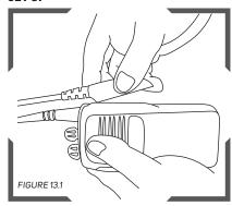
Connect the PTT Cable to the Hand Set depending on the type used.
