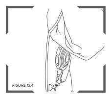
To operate the device, press your elbow onto the PTT Button, and then speak.
