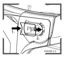
Do the same thing on the other side to fully secure the lens and the hood to the Helmet.
