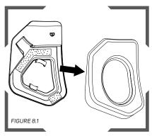
Remove the side pads from the covers that are attached withhook and loop.
