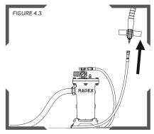
Now connect the Breathing Air Supply Hose to the Flow Control Device. Air should be now flowing through the Respirator.
