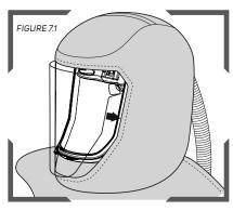
Peel off the backing of the cassette lenses and apply the lenses to the outside of the lens sewn into the hood.
