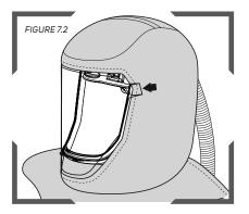
Use the folded over tabs to remove each lens as needed.
