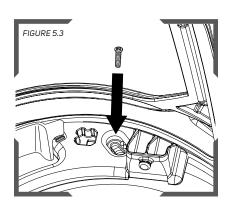
The position of the head harness can be adjusted by loosening the screws that hold the front bracket and sliding it forward or backwards into the desired slot. Once in position, tighten the screws.
