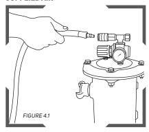
Connect the Breathing Air Supply Hose to the point of attachment (04-900 Radex® Airline Filter) shown.
