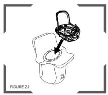
Insert the helmet into the hood with front of the Helmet towards the lens of the hood.
