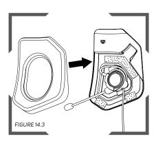
Attach the side pad back onto the cover over the Communication. Insert the side pad back into the helmet.
