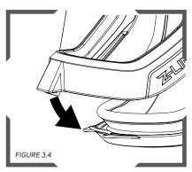
Close the visor making sure it LATCHES SECURELY to the front of the jaw. Listen for the visor latching over the tab on the front of the jaw.
