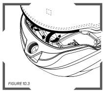
Then secure the hook and loop strips through the attachment points in the back of the helmet. These should be tight enough so that when the rear seal is pressed in, the fabric is bunched up a little.
