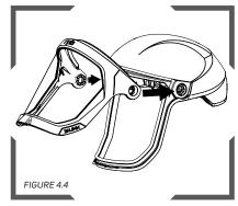
Place the visor onto the helmet pivot points, insert the pivot pins and springs, then screw in the attachment screws from the inside of the helmet until tight.
