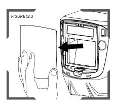
Remove the Impact Lens by squeezing together the sides of the Impact Lens. If just replacing the Impact Lens, then place the new Impact Lens in and replace the green ADF Retainer.
