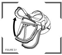
To replace the Safety Lens, lift up the visor, unlatch the inner visor from the outer visor and open them apart.
