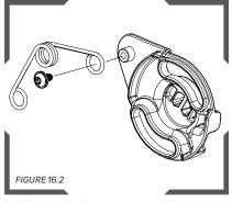
Position the spring onto the new flip up mechanism and secure it with the screw provided.
