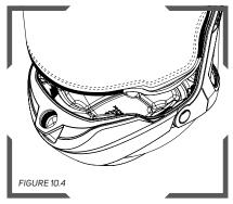
Press the rubber seal on the cape or face seal into the track that goes around the back of the helmet, making sure the cape/face seal is completely attached all of the way around. When the back of the cape is tugged on, the strips should keep it from coming out of the track.
