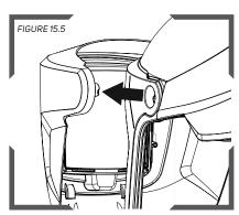
To remove the Welding Visor from the Z-LINK®, pull the sides of the Welding Visor out until the connection sockets snap out of the Pivot Pins in the Z-LINK®. This can also be done while wearing the Z-LINK®.
