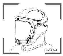
When using a face seal, make sure the elastic edge is under the users chin at the front and is in contact all of the way around the neck and back of the head.
