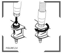
Connect the Breathing Tube to the flow control device.
