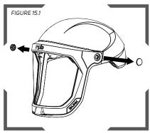
To install the Z-LINK® Welding Visor, remove the pivot pin caps on the Z-LINK®.
