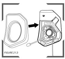
Attach the side pad back onto the cover over the Communication.
