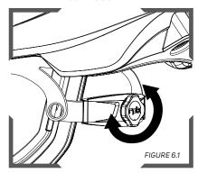
The head harness can be tightened or loosened using the ratchet knob on the back of the headband.
