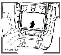
To install the magnifying lens for welding, slide the lens up into the brackets at an angle until it is securely in the brackets.
