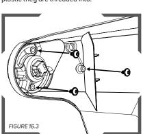
Carefully align the replacement spring and the flip-up mechanism onto the pegs in the Welding Visor. Insert and screw in the 3 replacement screws to attach the spring and mechanism without over tightening.
