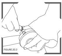
Connect the PTT cable to the head set cable and place the cable underneath the cape.
