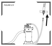
Now connect the Breathing Air Supply Hose to the Flow Control Device. Air should be now flowing through the Respirator.
