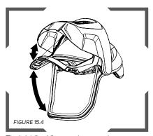
The Welding Visor can be rotated up independently of the Visor or together with the Visor.
