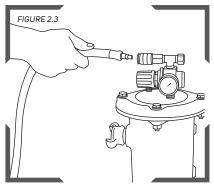
Connect the Breathing Air Supply Hose to the point of attachment (04-900 Radex® Airline Filter) shown.
