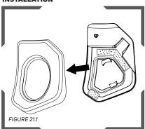
Remove the side pad from the cover that is attached with hook and loop on the side of the helmet that the Communication is to be installed. The Communication can be installed on either side of the helmet.
