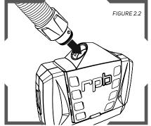
Insert the bayonet end of the breathing tube into the outlet of the PX4 AIR® PAPR and twist it in until it is secure.
