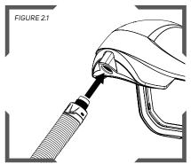
Insert the threaded end of the breathing tube (O4-835) into the threaded hole in the back of the Z-LINK® and screw the breathing tube in completely without over tightening.
