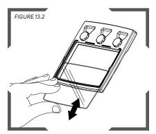
To replace the Rear ADF Lens, slide the lens out and replace it with a new one.
