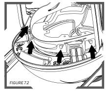
Replace the brow pad by placing the holes on one side over the hooks on the head harness and then wrap the pad over the top of the head harness. Stretch the pad around the bottom of the head harness and secure the holes over the hooks.
