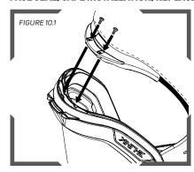
To install the cape or face seal, start by inserting the front clip into the track around the front of the jaw. Make sure the holes are aligned and insert and tighten the screw to secure the front of the cape. Press the rubber seal in up both sides.
