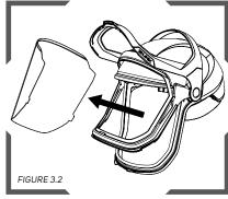
Pull out the lens and insert a new Safety Lens making sure the tabs of the lens are in all four attachment points on the visor and the lens is inside of the guide along the bottom front edge of the visor.
