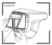
To remove the ADF, push down on the tab at the bottom of the ADF to release it and pull the ADF out.
