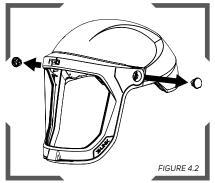
Remove the cap, pivot pin, and spring from the visor on both sides. Pull the visor out of the pivot points and remove from the helmet.
