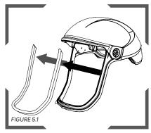
The visor seal can be replaced by pulling it out of the track around the visor opening.
