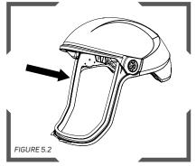
Starting from one of the top corners, insert the new visor seal by pressing the edge into the track all of the way around the visor opening.
