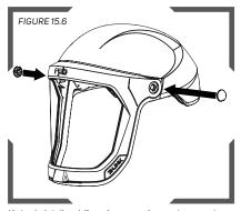
If the Welding Visor is not going to be used again for a while, the socket caps can be snapped back into the Pivot Pins to keep the area free of debris.
