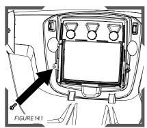
With the screws supplied, screw the left lens bracket into place by tightening the screws firmly without over tightening. Then screw in the right bracket.
