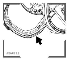
Close the outer visor over inner visor and lens, making sure the latches at the corners are secure.
