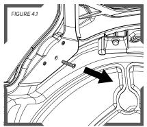
To replace the Visor, from inside of the helmet, unscrew the center screw from the visor pivot point on each side.
