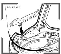
Next attach the side cape clips into the helmet. Make sure the clip goes over the notch on the helmet and the clip edge goes into the track around the edge of the helmet.
