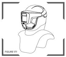
When welding, be sure to install a RPB® Zytec face seal or shoulder cape for adequate protection from sparks, debris, and light flashes. If using a face seal, make sure all skin, such as the neck, is covered to prevent UV radiation and burns. Follow the cape installation instructions on page 23.
