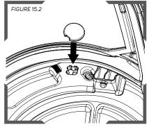
Insert the caps into the holding sockets on the Head Harness Bracket so they don't get lost while using the Welding Visor.
