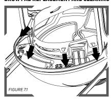
To remove the brow pad, stretch the brow pad over the hooks on the head harness and take it off. Clean it with mild detergent or replace it with a new one.
