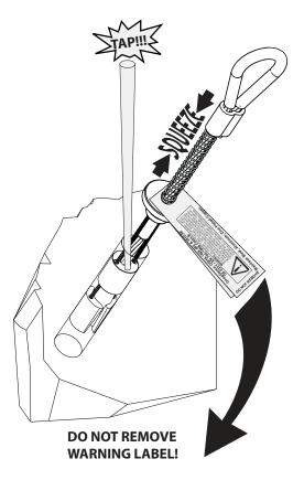
May be used as an anchor point for a leading edge restraint system. See optional anchor points below for example. The use of two anchors is not required for leading edge restraint systems unless otherwise specified by the manufacturer.
