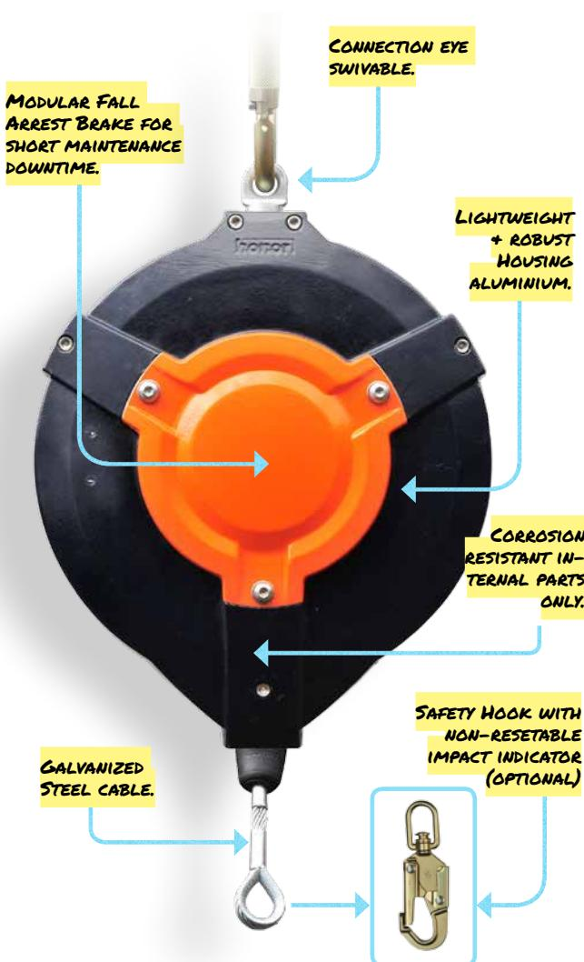
With max. 33 meters (LA33/300) cable length. Used as a backup device to the main support unit, the load arrestor's inertia locking mechanism will engage stopping the load if it breaks free.
