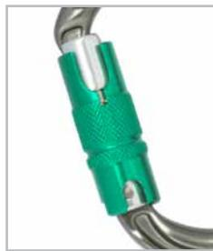
**Durolock:** (Dual Rotor Lock) was designed to minimize the chances to accidental gate opening, and maximize levels of security. Its complex, yet easy to manipulate gate requires four (!) distinct actions to open, and once released, automatically returns to the locked position. It is perfect for complex safety applications.
