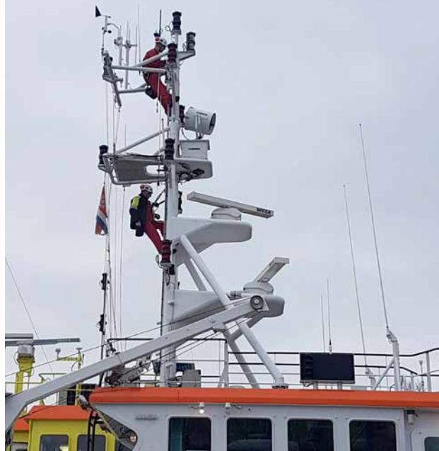
Every rail system is fitted with hand operated entry and exit securities. Also an Extension Bracket can be mounted on the top end of the rail to extend the rail from a manhole, surface level or to enter a roof.
