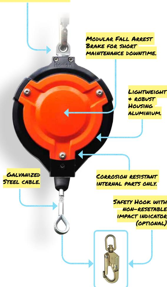
With max. 15 meters (LA15/300) cable length. Used as a backup device to the main support unit, the load arrestor's inertia locking mechanism will engage stopping the load if it breaks free.
