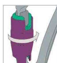
1. Turn outer barrel anticlockwise.
