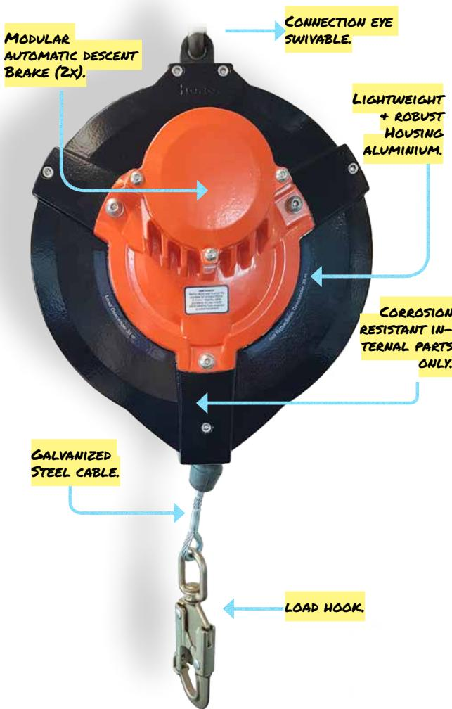
With max. 33 meters (LAD33/200) cable length. Used as a backup device to the main support unit, the load arrestor's inertia locking mechanism will engage stopping the load if it breaks free.
