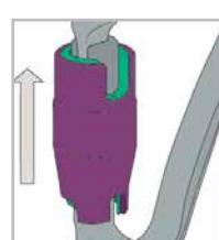
2. Push outer barrel upwards
