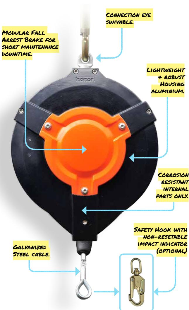
With max. 15 meters (LA15/500) cable length. Used as a backup device to the main support unit, the load arrestor's inertia locking mechanism will engage stopping the load if it breaks free.
