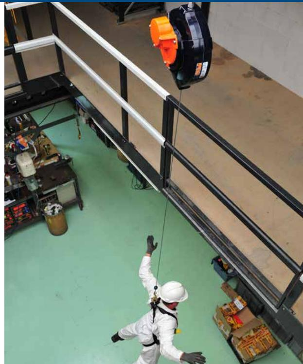
This unique descender is a very important if self rescue is needed. PED15 devices are available with galvanized steel wire ropes.
