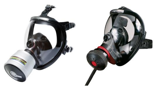
Extra wide view full face mask complying to European norms EN 136. One size fits all. For use with dust, gas and combined filters with a threaded connector conforming to EN 148/1 and an overpressure version for use with compressed air supply devices (with threaded connector according to EN 148/3). All versions are available in EPDM and silicone rubber.
