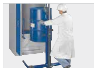
Drum lifter for picking up and transporting 200 l (52.83 gal) drums. Ideally used with heavy load drawer.
