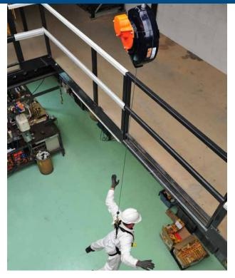
This unique descender is a very important if self rescue Is needed. PED15 devices are available with galvanized steel wire ropes.
