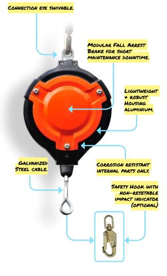
With max. 15 meters (LA15/300) cable length. Used as a backup device to the main support unit, the load arrestor's intertia locking mechanism will engage stopping the load if it breaks free.
