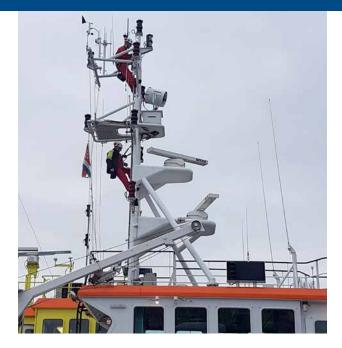
Every rail system is fitted with hand operated entry and exit securities. Also an Extension Bracket can be mounted on the top end of the rail to extend the rail from a manhole, surface level or to enter a roof.
