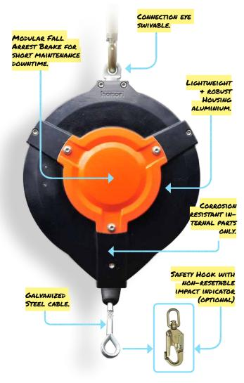
With max. 33 meters (LA33/300) cable length. Used as a backup device to the main support unit, the load arrestor's intertia locking mechanism will engage stopping the load if it breaks free.
