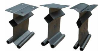
Deformed Intermediate Bracket
