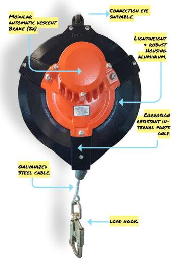
With max. 33 meters (LAD33/200) cable length. Used as a backup device to the main support unit, the load arrestor's intertia locking mechanism will engage stopping the load if it breaks free.
