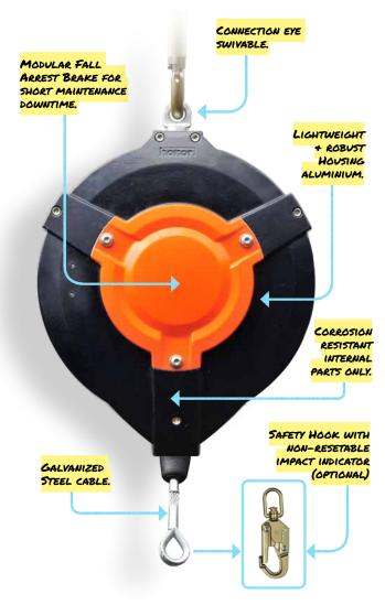
With max. 15 meters (LA15/500) cable length. Used as a backup device to the main support unit, the load arrestor's intertia locking mechanism will engage stopping the load if it breaks free.
