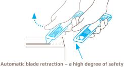
The automatic blade retraction of the SECUNORM 500 guarantees a high degree of safety from cut injuries. As soon as you have started to cut, take your thumb off the slider. Then the blade will retract into the handle immediately after leaving the material being cut.
