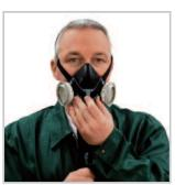
Pull down front straps and lock lever
