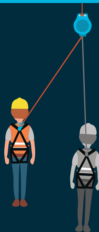
Figure 2 - Illustrates sideways impact with an adjacent vertical structure.
