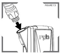
Take the bayonet end, insert the connection into the PX5® and make sure the slots line up with the pegs in the PX5® outlet.
