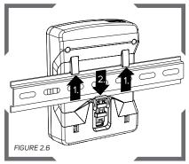
Hook the battery charger using the small tabs on the back over the top edge of the DIN rail (1.) and then rotate it down until it clicks over the bottom edge of the DIN rail (2.). The bottom tab should return to the resting location. Pull gently to test.
