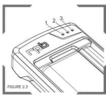
Follow the indicator lights on the top right corner of the charging station to know the status of the charge process. 1 blinking LED = low charge. 2 blinking LEDs = medium charge, 3 blinking LEDs = high charge, 3 solid LEDs = fully charged, approx. 95-100% charged.
