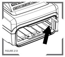
Remove the battery door, then slide the hinge back into the unit to remove it from the track inside of the battery compartment.
