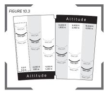
The flow meter levels are grouped by temperature and altitude. Ex.: dashed box shows levels for different temps at Oft above sea level. Choose the altitude closest to the altitude where the check is being performed.
