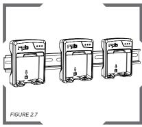
If required, multiple chargers can be mounted onto the DIN rail as per figure 2.6.
