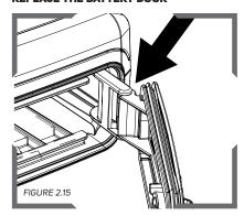
Disconnect the door from the hinge by pulling the door in the direction of the hinge opening. Attach the new door by snapping the door onto the hinge cross bar.
