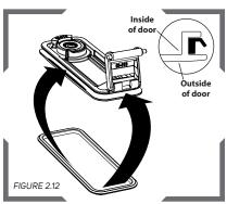
With the battery door off or open, remove the old seal. Note the orientation of the lip on the seal. Place the new seal into position by stretching it around the door, into the channel around the edge of the door.
