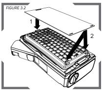
The prefilter can be attached to the HE Filter before or after the filters are installed onto the PAPR. Secure the prefilter onto the top tab (1.) on the HE filter and then over the bottom tabs (2.) on the bottom of the HE filter.
