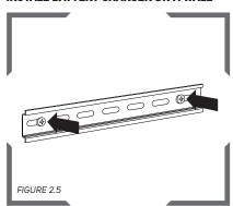
Using a desired length of DIN rail, depending on how many chargers you want to mount to it. Screw the DIN rail into the desired location for charging. Ensure the location of this mount meets those specified in the recommendations on page 11.
