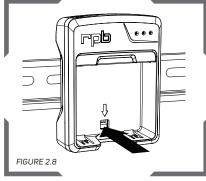
Remove the charger from the DIN rail using a flat head screw driver. Pull down the tab inside the cutout in the charger to release the clip from the DIN rail. Pull the charger from the DIN rail at the bottom and then lift the charger off.
