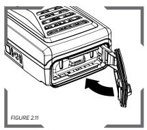
Close the battery compartment door, making sure the seal around the door properly seats and the latch securely engages. The door must be completely closed and sealed for the IP 65 rating and to protect the unit from damage from liquids or debris.
