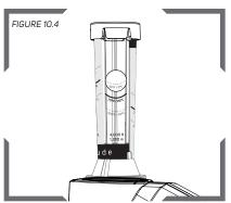
When the PX5° is on speed 1, the ball will float inside the flow meter. Ensure that it sits above the curved line for the altitude and temp for where the check is being performed. Ex: 4,000ft above sea level and 70°F.
