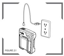
Connect the power cord to the charging station. Connect the other end of the power cord to the electrical source (110-240v).
