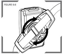
Following the "lock" and "unlock" symbols with the arrow on the belt bracket. Rotate the bracket until the tab clicks over the raised ramp on the back of the PX5®. Check that it is secure.
