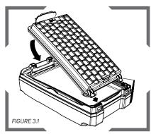
Mount the O3-892 HE Filter into the PX5° by placing the tabs through the slots in the top edge of the PX5° filter area and rotate the filter down until the bottom tab snaps into place. Check that both tabs on the filter latch are secure.
