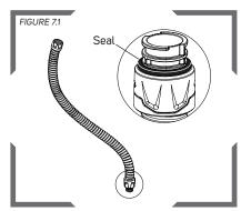
Inspect the breathing tube (04-831) and ensure there is no damage and that the o-rings are in place and in good condition.
