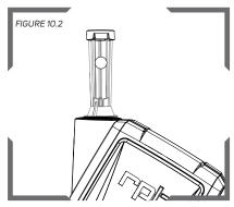
Turn the PX5® unit on and then orientate the unit so the flow meter is pointing straight up or vertical to achieve the most accurate results.
