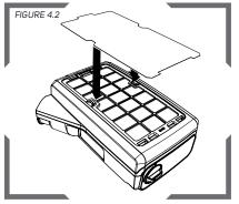
Place the filter door back onto the the PX5°. Secure the spark arrestor under the tabs on the front of the filter door.
