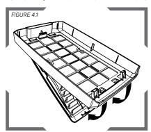
Remove the green spark arrester cover by removing the filter door and then pushing up on the tabs that hold the spark arrester cover in place.
