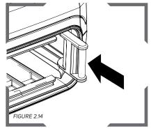
Slide the new hinge into the battery compartment with the pegs on the hinge in the tracks. Then snap the battery door onto the hinge crossbar.
