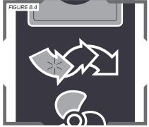
Filter blockage is indicated on the User Interface Panel by the multi-colored arrow under the power button. Green = full airflow, Yellow = mild blockage, reduced airflow, Red = blocked airflow. When the Red arrow is lit, safely exit the work area and check for any blockages in the air path. If blockage is not resolved, follow the filter change instructions.
