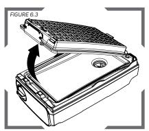
Remove the filter from the PX5® by pressing on the tab at the bottom end of the filter and lift up. Dispose of it in a responsible and safe manor in accordance with regulations. Install new filter and inspect/replace 03-890 prefilter.
