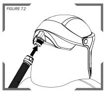
Screw the threaded end onto the inlet of the respirator.
