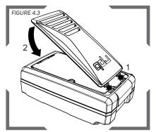
Reattach the spark arrester cover by rotating the tabs on the top into the slots in the filter door (1). Rotate the cover down until it clips in securely at the bottom (2).
