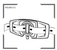
Thread the belt through the belt bracket as shown above, note the orientation.
