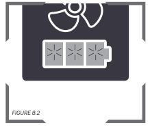
The battery level is indicated by the battery shaped LED panels on the side of the PX5°. 3 green LEDs = fully charged, 2 green LEDs = 25-75% charged, 1 green LED = less than 25% charged, 1 red LED blinking = 5% or less charge remaining, the battery needs to be charged and is about to turn off.
