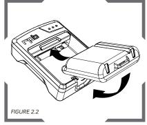
Fit the battery into the charging station by sliding the top of the battery into the charger housing and then rotate the battery down until it clicks into place.
