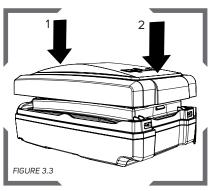
Orient the filter door with the handle cutout towards the top, opposite the battery door. Reattach the filter door by placing the door over the unit with filter in place and pressing on top (1) and bottom (2) until firm. You should hear a click and there should be little to no gap visible when clipped.
