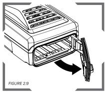
To insert the battery into the PX5®, open the battery compartment door on the bottom of the unit by twisting the knob to "unlocked".
