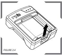
To remove the battery from the charging station, grip the charger housing firmly if not fixed in place, pull up on the tab on the bottom of the battery and slide the battery from the charger housing.
