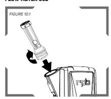
Insert the flow meter into the air outlet. Line up the bayonet slots and turn clockwise 1/2 turn until it locks into place.
