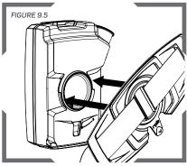
Line up the circular slots of the bracket with the tabs on the back of the PX5°. The locking tab on the belt bracket should be facing towards the bottom.
