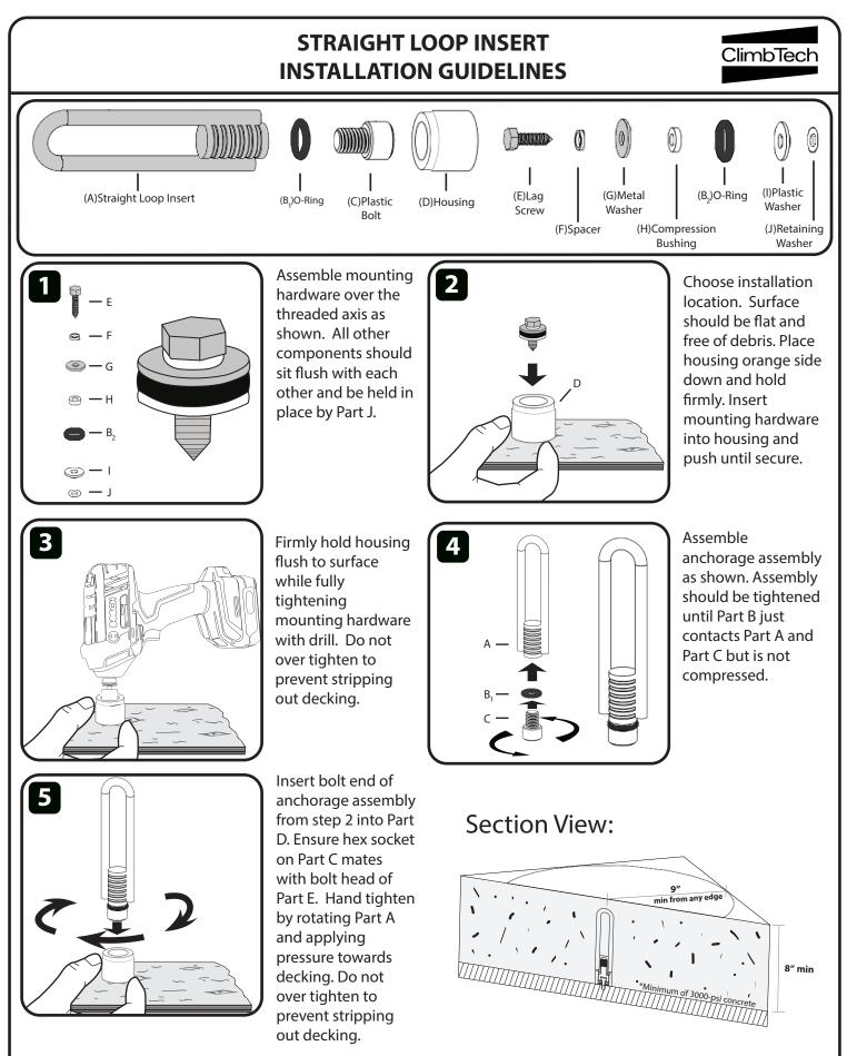
\*Note: Avoid kicking or knocking over installed Straight Loop Inserts while working. It is recommended that inserts are fastened to rebar by wire tie or equivalent method for additional support.
