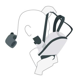
Turn power unit on. NOTE the motor and air will not flow until the respirator is donned and has detected breathing. Place the power unit at the back of the neck and clip on to the full face mask on both sides. Start breathing. The motor and air flow should start.
