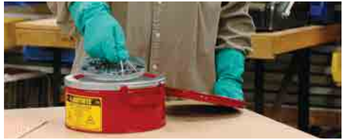
Clean small parts by pushing down dasher plate and agitate in cleaning solvent.
