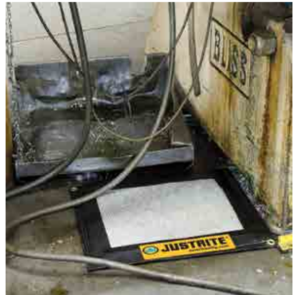
Position drip pad in tight spaces between machinery to capture oily leaks.
