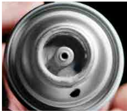
Smooth side puncture leaves no jagged edges.
