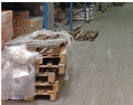
Clutter in aisles or walkways create trip hazards.
